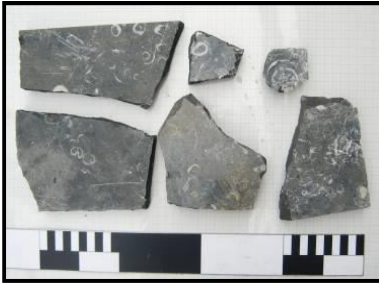
Figure 13: Wenlock-type oolitic limestone from the West Yard, National Trust
