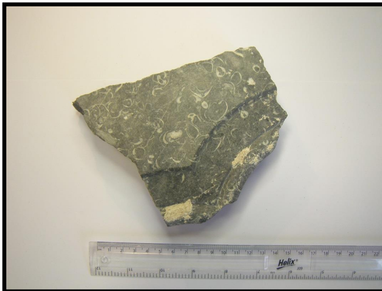
Figure 14: Wenlock-type oolitic limestone from the Queen Anne House at Castle Ward
