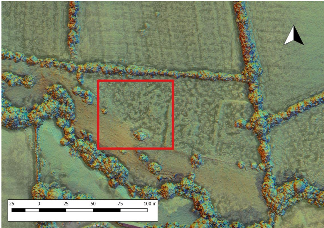
Figure 3 Area to be surveyed. Drone sourced combined semi-transparent image utilising the orthomosaic, a multi-directional hillshade and Local Dominance overlays
