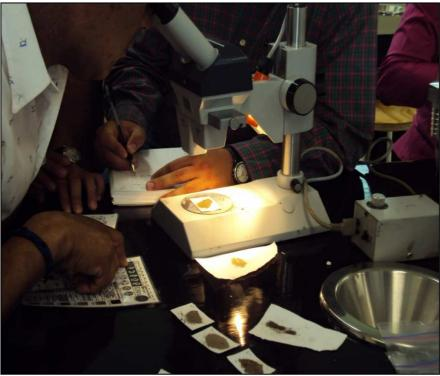
Figure. 2. Practice in the lab with stereo micrscopy, Munsell chart, the geotechnical gauge and table from Powers and Krumbein
