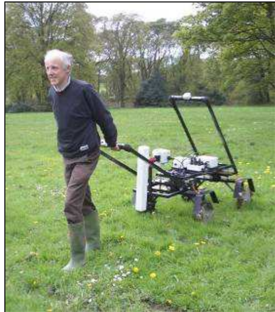
Fig 1. (Left) FM256 Fluxgate Gradiometer and (right) MSP40 Mobile Sensor Platform with FM256 for combined resistance and magnetic surveys.
