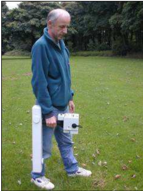
Fig 1. (Left) FM256 Fluxgate Gradiometer and (right) MSP40 Mobile Sensor Platform with FM256 for combined resistance and magnetic surveys.
