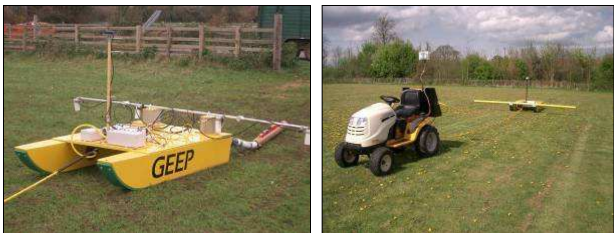
Fig. 1. (Left) Geophysical Exploration Equipment Platform (GEEP) multi-sensor platform from Geomatrix showing configurations with 4 caesium vapour magnetometers EM38 installed and (right) Dual-EM, multi-depth system.
