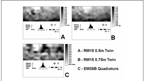
*Figure 1*: Belhuish House, Dorset. Comparison of RM-15 0.5m and 0.75m twin results with the EM38B quadrature phase results displayed as resistivity. Note the low resistance anomaly one third of the way along the top side of the survey area that corresponds to the position of the known animal grave from 2001.
