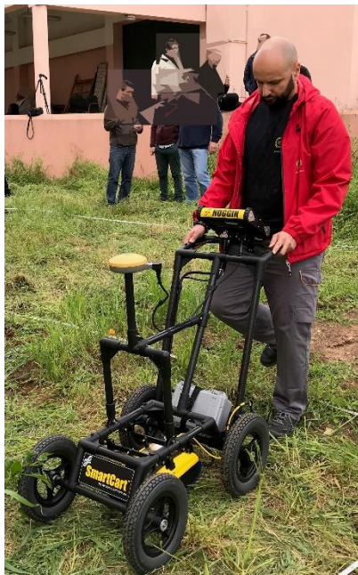
Prof Pier Matteo Barone, using Ground Penetrating Radar (Photos: Pier Matteo Barone)
