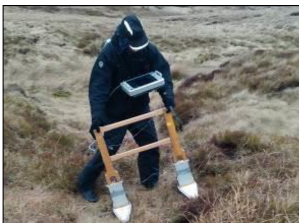
Laurance Donnelly and Alastair Ruffell conducted experimental GPR over a suspect homicide grave in Northern Europe
