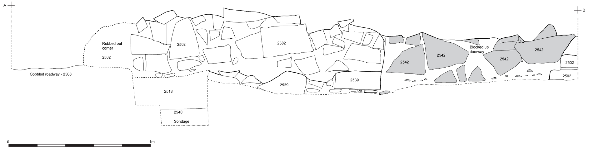
Figure 81: Trench 25a, west facing elevation of wall 2502 and blocked-up doorway 2542
