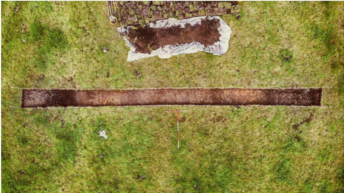
Figure 6: Aerial view of the trench excavated across “The Line” showing its clay surface, the “soling” or platform on which the stone roadway would have been set had the road been completed (Ryan Montgomery).
